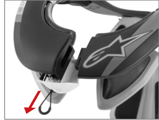
Figure 2 – Quick Release Locking System: rapid and efficient fitting/removal, which offers a secure and convenient attachment which can also be quickly opened in case of emergency.
